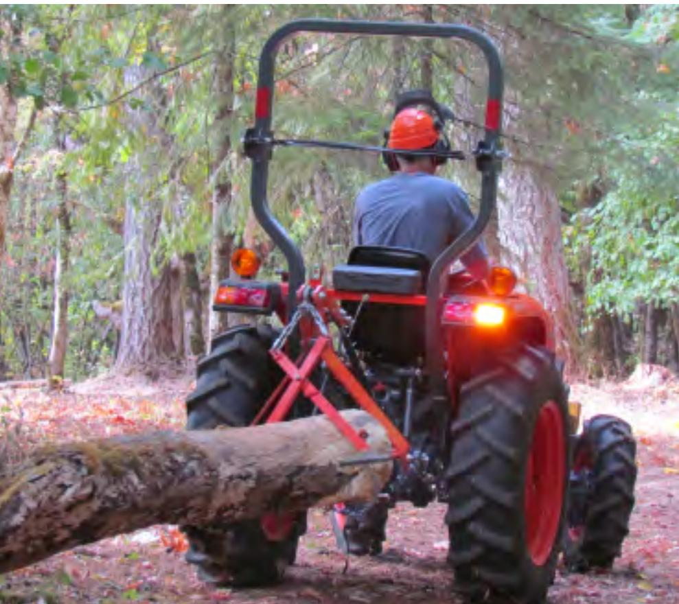
With the tongs in place, the skidder provides secure control over the butt of the log and away it goes.
