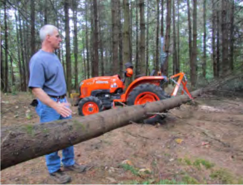
When processing firewood, the operator moves the skidder to the center of this green Douglas fir, where he easily suspends it at a comfortable height that allows him to buck it while standing comfortably upright and without digging his chain bar in the dirt.
